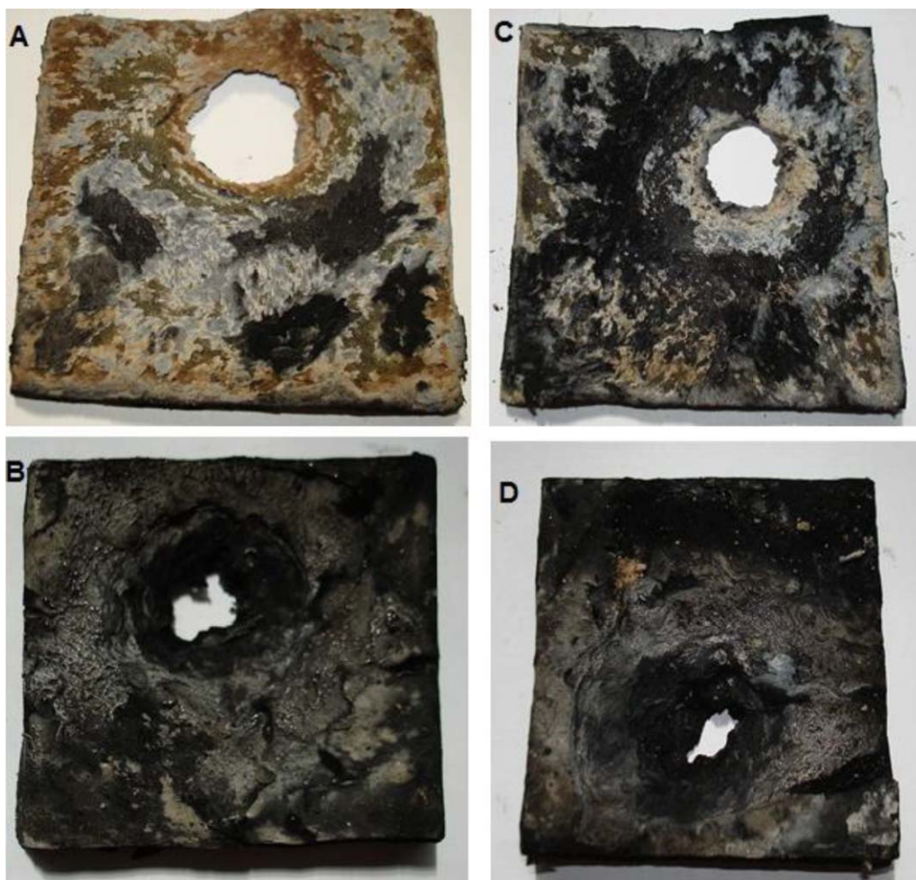
Figure 9. Comparison of the ablation pit for burnt materials of (a) Kev20, (b) Kev20BX20, (c) CF20, and (d) CF20BX20. [Color figure can be viewed in the online issue, which is available at wileyonlinelibrary.com .]
